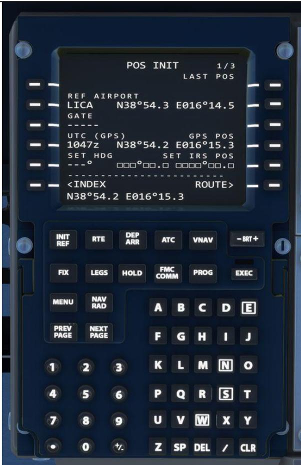
The POS INIT page Using the FMC keyboard, enter KTNT then press the LSK 2L key and we'll see it appear under the REF airport. Also, check that the clock on 5L matches the correct time. Then press LSK 6R to go to the ROUTE page.
